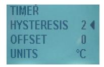
The hysteresis is the temperature difference (in degrees) between the point at which the heating switches off and switches on again. The heating will always switch off at the programmed set point and will switch back on at the set point minus the hysteresis value. The hysteresis range is 1 to 9 with a default value of 5
