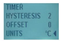
Whilst the arrow on the screen points to the Units option, you can use the  $\triangle$  or  $\nabla$  keys to toggle the setting between C (Celsius) and F (Fahrenheit).
